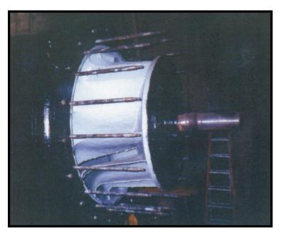
The turbine was dismantled and all metal surfaces were abrasive blasted to SA2 1/2.
