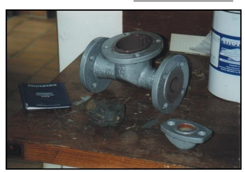
The valves were first of all cleaned and prepared. The insides were rebuilt where required using Cerami-Tech EG and the entire internal surface coated with Cerami-Tech FG. The outside of the valves were coated with Corro-Tech GP and Chemi-Tech EP.
