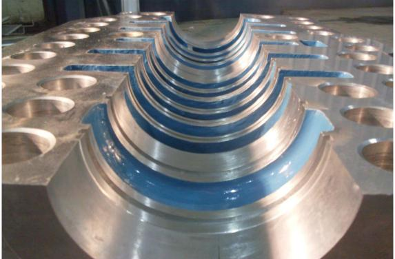
From the practice application which shows that the Ceramic coating protect the equipment successfully.
